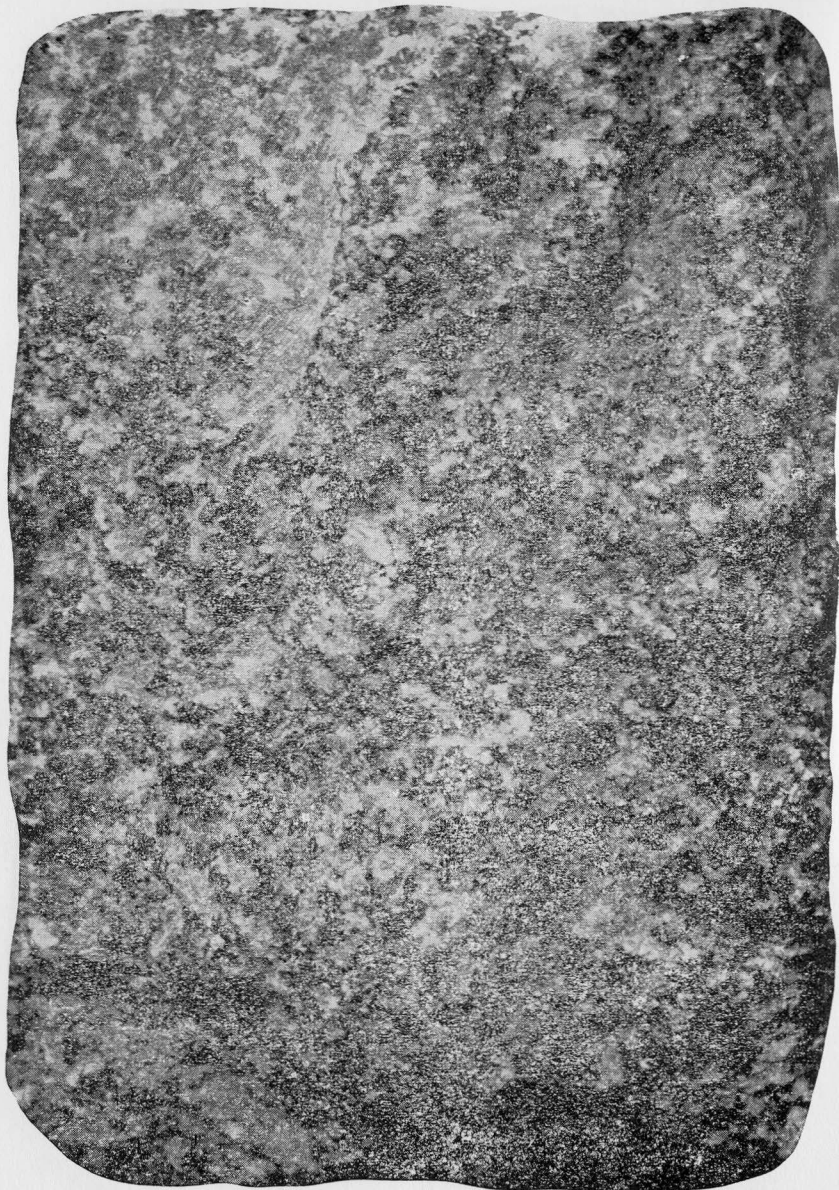
PLATE 2. Medium-grained biotite-hornblende diorite exhibiting hypidiomorphic-granular texture. Color index about 40. (x2)
