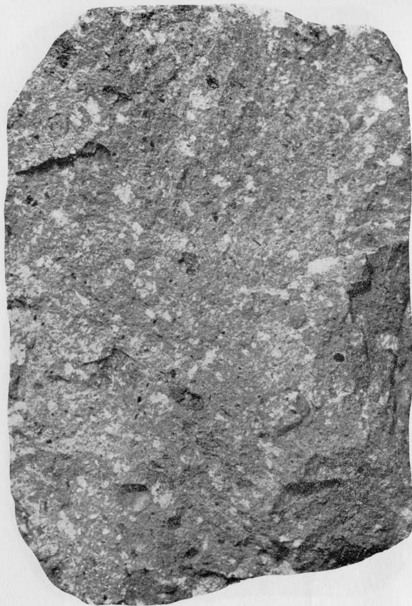
PLATE 11. Dacite porphyry. Round phenocrysts of quartz and white lath-shaped phenocrysts of plagioclase in gray aphanitic groundmass. (x3)
