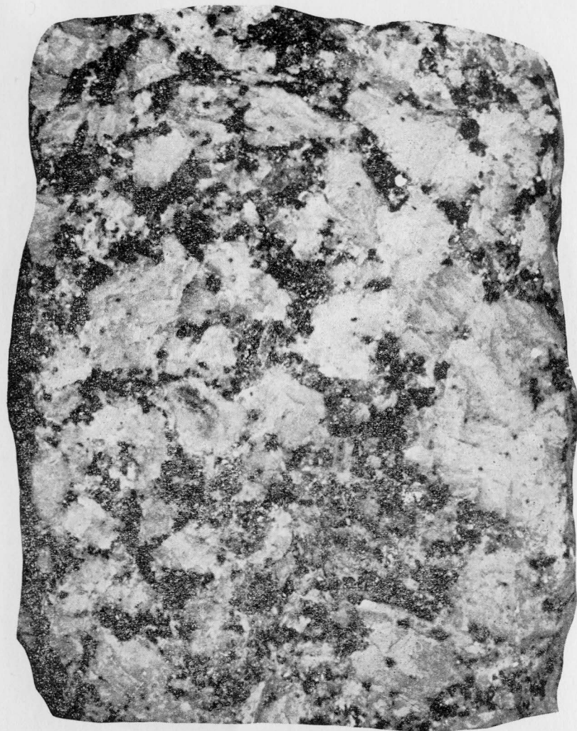
PLATE 7. Medium-grained hornblende-biotite quartz monzonite porphyry. Large pale-colored grains of orthoclase set in a groundmass of quartz, plagioclase, biotite and hornblende. Color index about 10. ( \times 1\frac{1}{2} )
