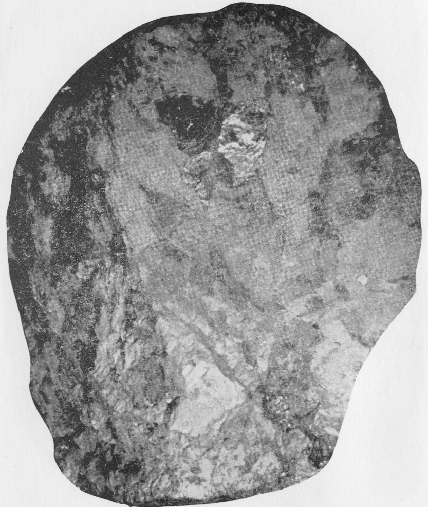
PLATE 9. Granite pegmatite. Large grains of quartz, perthite, and biotite. (x \frac{1}{2} )
