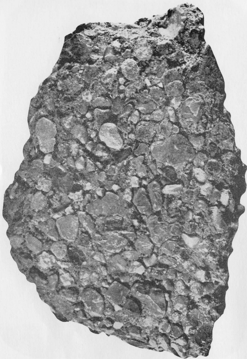
PLATE 16. Chert pebble conglomerate. A homogeneous conglomerate composed of pebbles of chert in a sand matrix. ( \times\frac{3}{4} ) (Photo by L. W. LeRoy)
