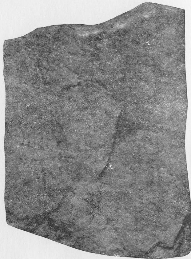
PLATE 21. Medium-grained orthoquartzite. Although the interstices of this specimen have been filled completely with authigenic quartz, the clastic texture is still vaguely visible. (x1)
