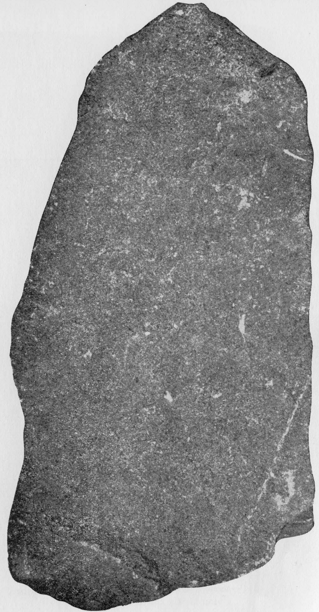
PLATE 23. Medium-grained graywacke. This specimen is dark olive green and as tough as fresh igneous rock. Megascopically visible are feldspar, rock fragments, minor quartz and a chloritic rock paste matrix. (x3)
