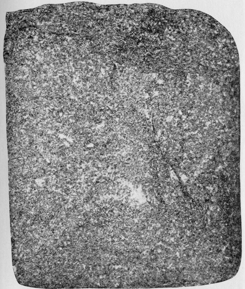
PLATE 3. Quartz diabase exhibiting diabasic texture. For magnified thin section see Plate 50. Color index about 60. (x1½)
