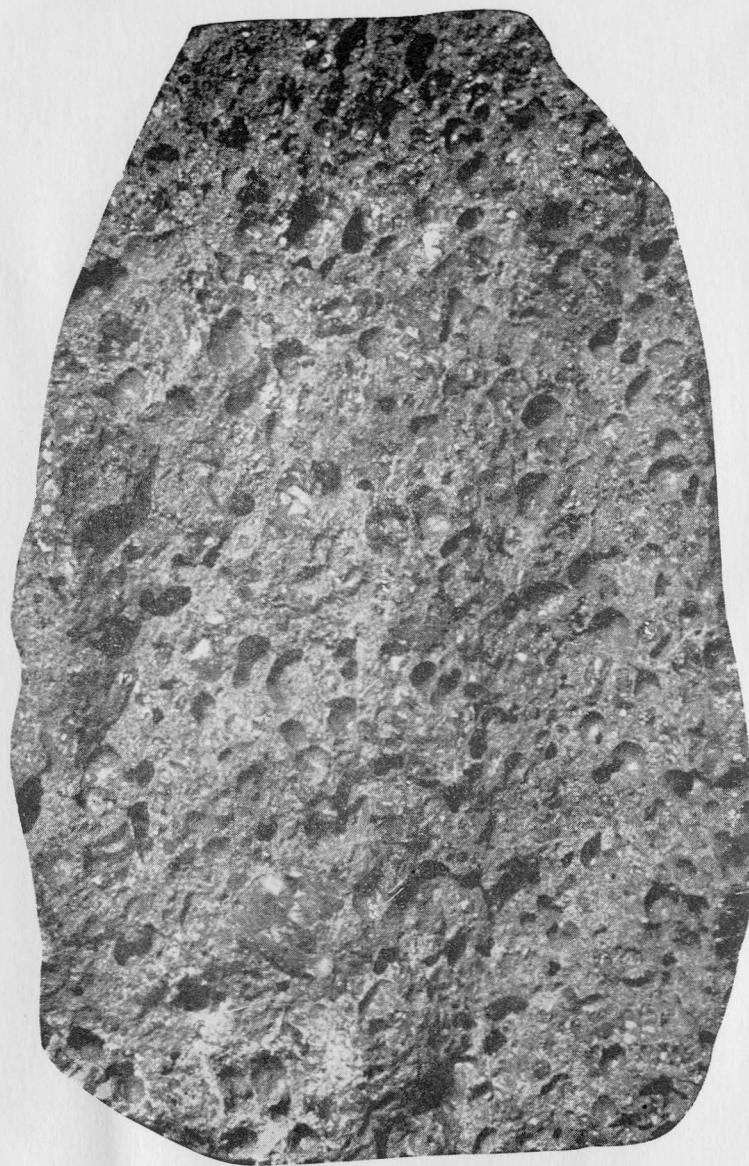
PLATE 13. Vesicular olivine trap porphyry (olivine basalt porphyry). Glassy phenocrysts are olivine. (x1)
