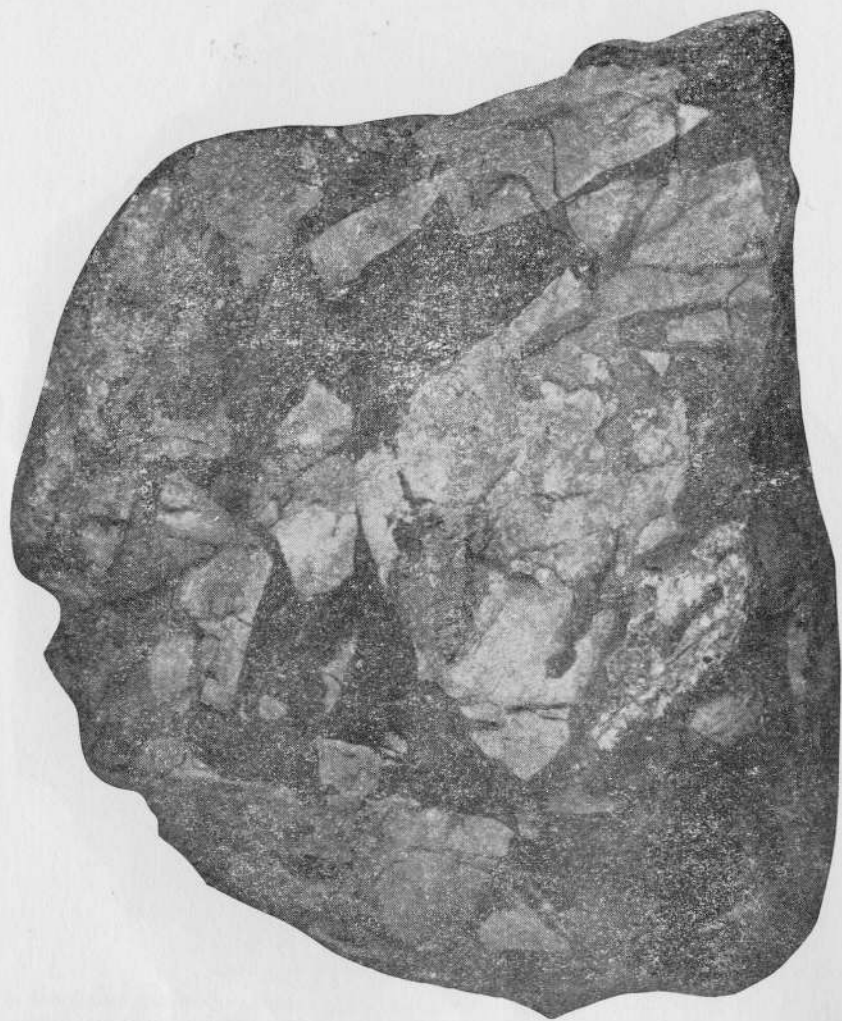
PLATE 18. Limestone breccia. A homogeneous breccia composed of pebble size fragments of limestone in a black siliceous matrix. ( \times\frac{1}{2} )
