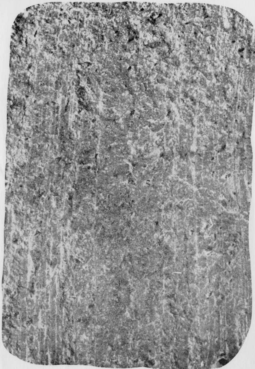
PLATE 14. Banded welded tuff with black phenocrysts of biotite and pale, inconspicuous phenocrysts of quartz and sanidine. Pyroclastic texture is apparent only under the microscope. For magnified thin section see Plate 54. (x3)
