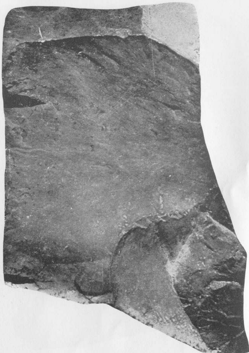
PLATE 25. Lithographic limestone. Note smooth aphanitic texture, giving conchoidal fracture. (x2)
