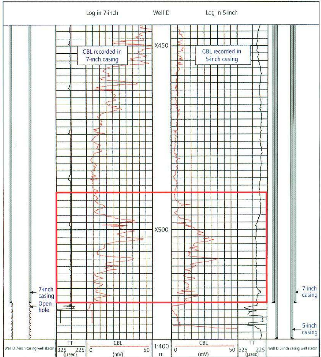
Figure 13.7 The CBL log was recorded inside the 7-inch casing and later in the 5-inch casing. Both logs show poor cement in the interval X520–X490 m (indicated by the red box), but in reality the cement between the 7-inch and 5-inch casings is good. In the latter case the poor cement between the 7-inch casing and the formation may be causing interference on the log. The transit time (TT) increase supports this theory
