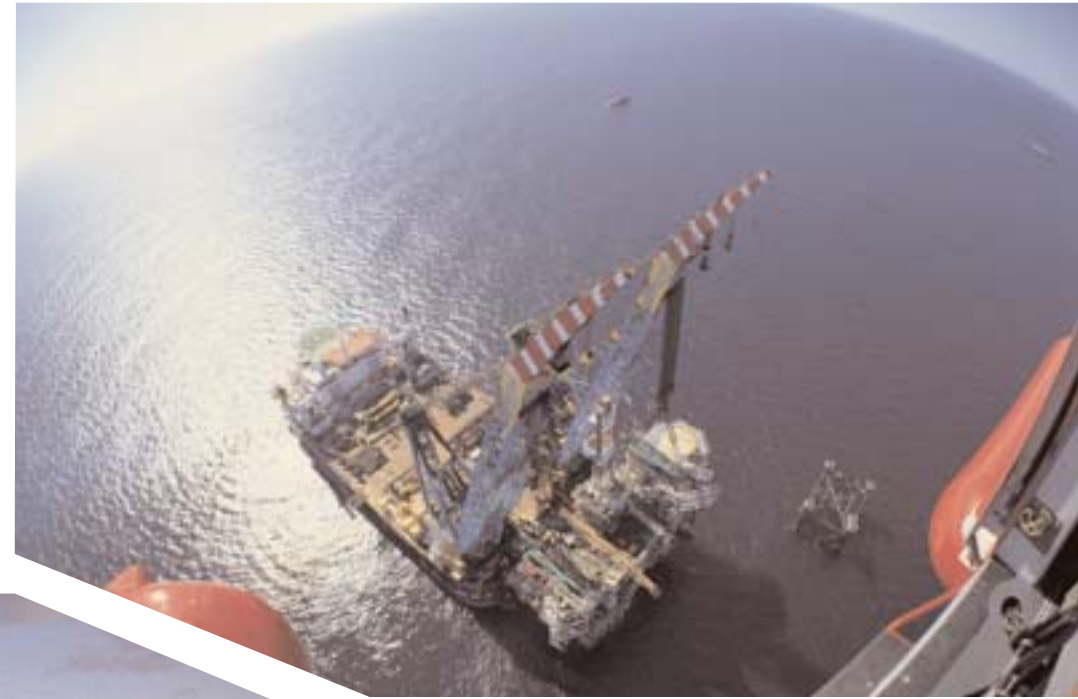
Saipem 7000, installation, World Heavy lift Record(10,400 tons) in DP, BP Andrew Field, North Sea, Off UK, 1996
